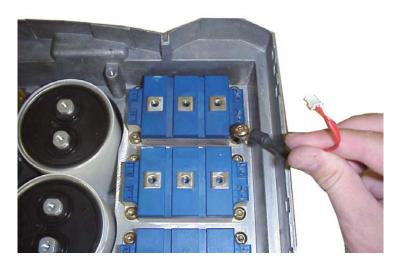
Remove and install the new thermistor
