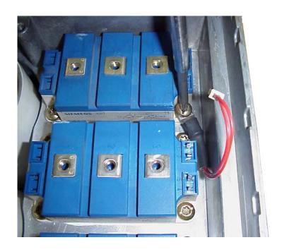
Use the T-30 Torx screwdriver to remove the thermistor.
